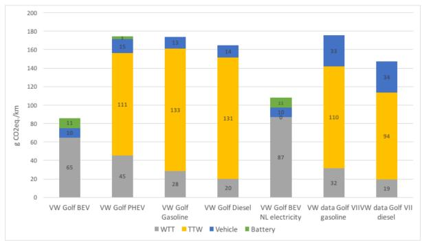
Figure 16 A <u>"Apples and pears comparison"</u> VW Golf (generation VII) GHG LCA emissions per kilometer comparing T31 model and VW LCA calculations ("VW data"); the example is to show the current difficulty in comparing LCA data as published, please NOTE: the T31 and VW data cannot be compared 1 to 1: VW uses a 150.000 km used as LCA unit, T31 200.000 km life time; VW uses the NEDC test results, T31 the RDE emissions
