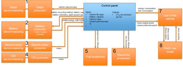
Figure 18 : Model structure and data exchange
