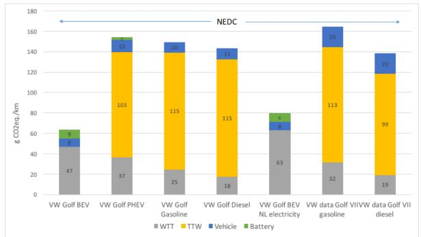
Figure 16 B <u>"Apples and apples comparison"</u> Comparison T31 VW Golf "NEDC" and VW data "NEDC": in this comparison, the data as provided by VW are aligned with the T31 data, for the VW data the life time km is adapted to 252.000 km and the T31 model has calculated the NEDC GHG emissions. Please note that as mentioned the T31 model does not "optimize" the NEDC results as do OEMs
