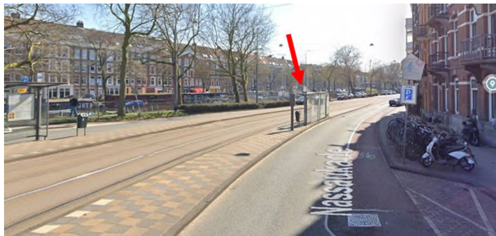
Figure 5: Bus stop on bend part of Nassaukade in Amsterdam can trigger false AEB reactions, as encountered during specific vehicle tests (image source: Google Street View)
