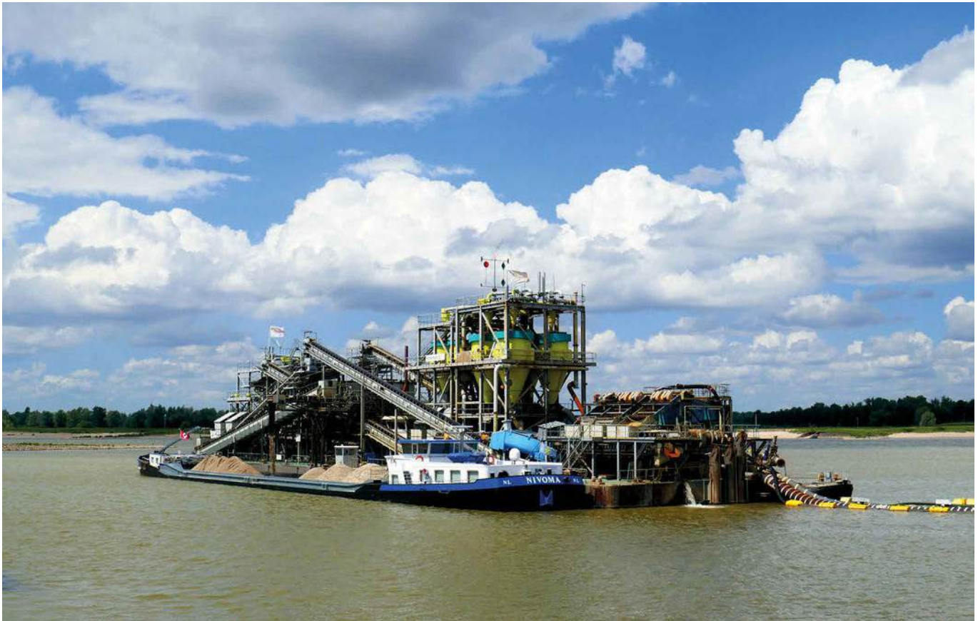
Figure 18.19. Floating aggregates classification unit (Geertjesgolf sandpit, Winssen, Netherlands). Photo by Rudolf Bak.
