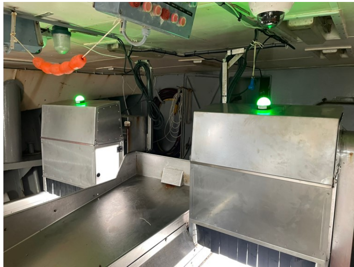
Figure 1. CatchWAM system. Concept (left) and two prototypes on board (right). Two systems are used because this vessel operated two conveyor belts to sort their catch.
