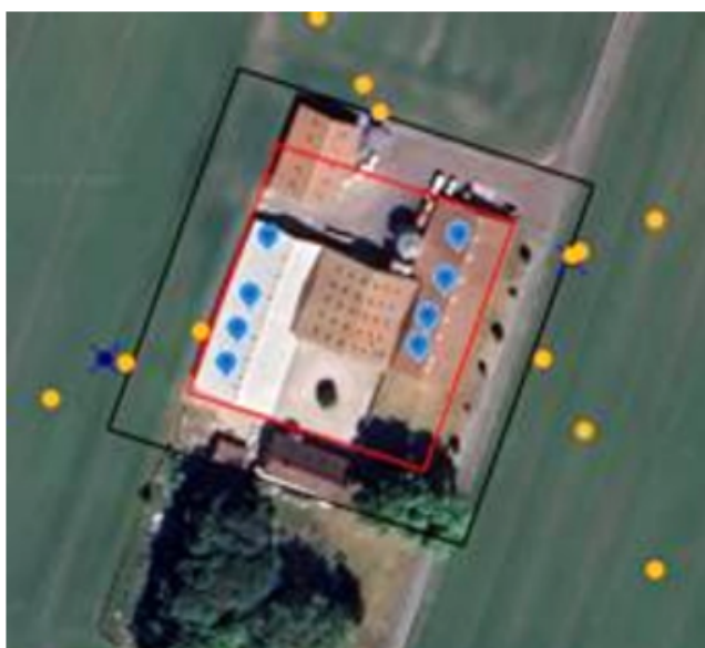
Figure 3.6 The measurement locations at the Ringsted farm closest to the building. A hypothetical rectangular building around the sources is shown in red. The receptor locations are shown as orange dots (deposition) and blue crosses (concentration). A 30 m buffer zone around the hypothetical building is shown in black in order to give an impression of dimensions.
