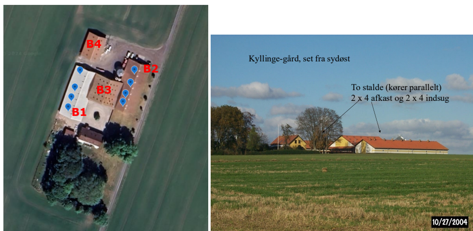
Figure 3.2 The poultry farm at Ringsted, On the left: Aerial picture of the farm taken from Google earth (accessed: 11-7-2024). The source locations have been marked by blue pins and the buildings have been marked from B1 – B4. On the right: a picture taken from the measurement campaign of the farm from the south-east. Provided to RIVM by Aarhus University.
