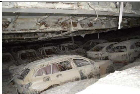
FIGURE 10B: 10 TH DECK BURNED CARS (Source: Physical inspection O/B - Fire Expert Report)
