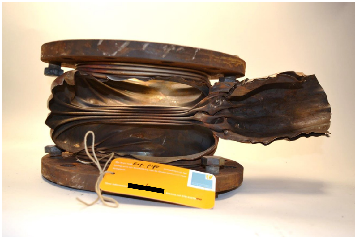
Figure 2. Overview of the fracture in the bellows with visibly expanded and compressed convolutions, the fractured double plate segment is still connected to the bellows.
