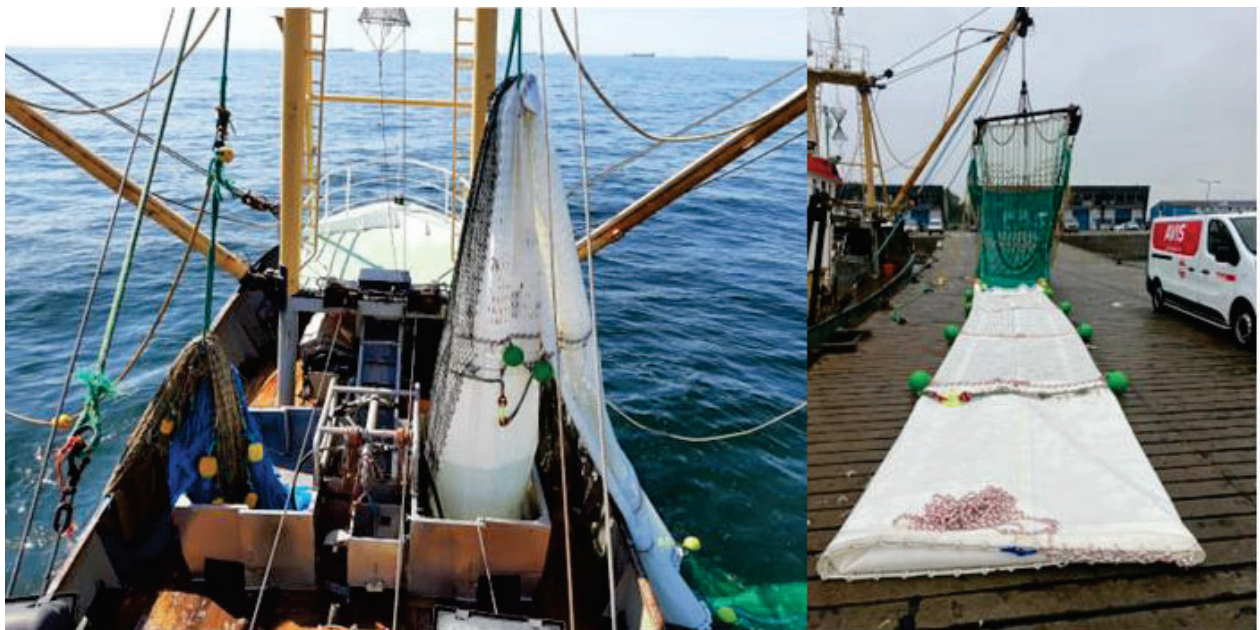
Figure 2. Kiwi-codend in use on starboard side of a Dutch beam trawler. Note the water retention in the lift bag module shown in the left hand image. Photo: Pieke Molenaar
