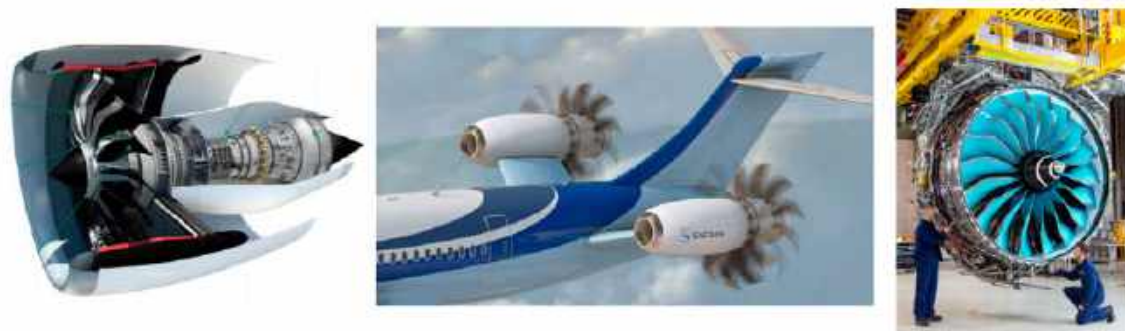
Figure 19: Clean Sky 2 engine technologies (Clean Sky 2 Technology Evaluator, 2021). From left to right: SAFRAN's Ultra-High Propulsion Efficiency (UHPE), SAFRAN's contra-rotating open rotors (CROR); Rolls Royce's Ultrafan (Rolls Royce, 2024)
