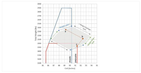
Figure 10: The centre of gravity limits for the normal and restricted categories (SE-KHF). (Source: Dutch Safety Board)
