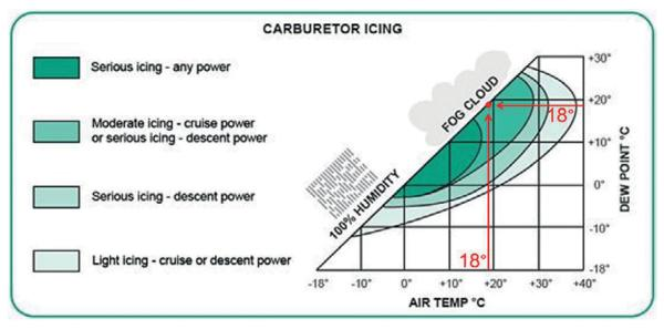
Figure 7: Carburettor icing prediction chart. (Source: Canadian Transportation Safety Board)
