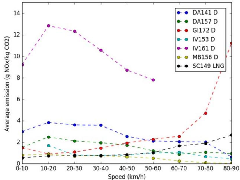
Figure 14: Speed binned emission data of NO<sub>x</sub> per kilogram of CO<sub>2</sub>. Vehicle IV161 is tested under worst case conditions which can't be regarded as fully representative, see paragraph 2.2.
