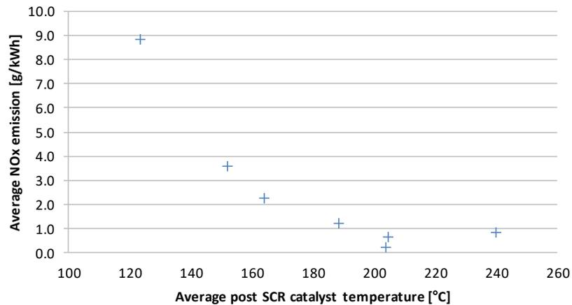
Figure 5: Average tail-pipe NO<sub>x</sub> emissions and post SCR catalyst temperature of seven of the tested diesel vehicles. Clearly, NO<sub>x</sub> emissions increase when the catalyst temperature decreases.
