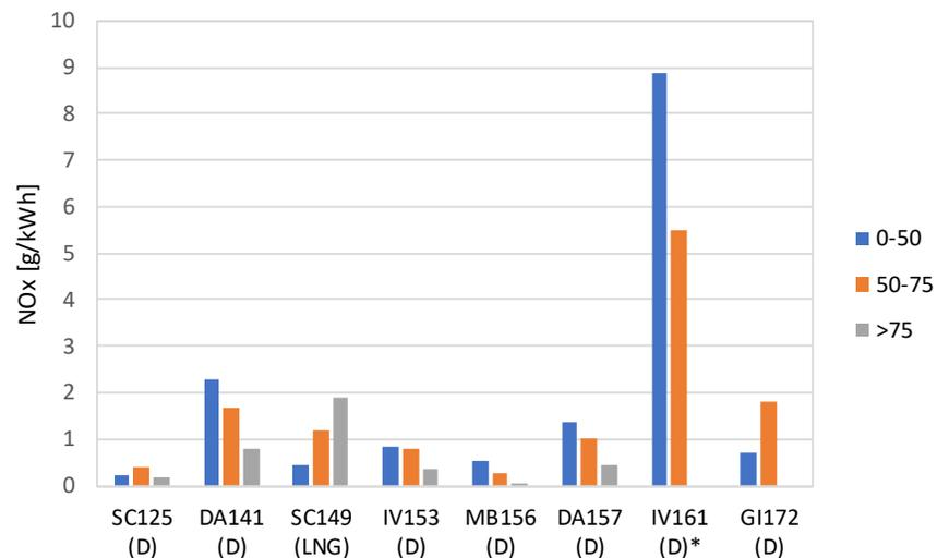
Figure 10: Average NO<sub>x</sub> emissions in g/kWh per speed range (in km/h). \*Vehicle IV161 is tested under worst case conditions which can't be regarded as full representative, see paragraph 2.2.
