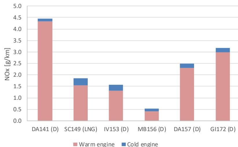
Figure 11: NO<sub>x</sub> emissions under cold and warm engine operation.
