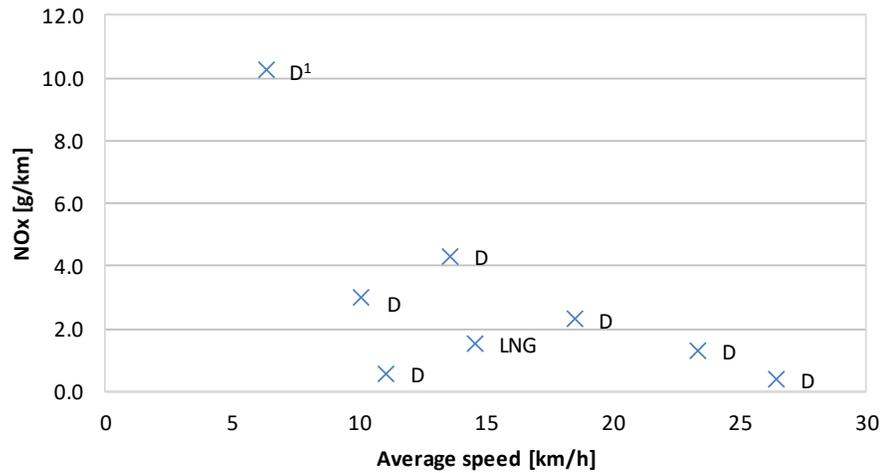
Figure 8: Average NO<sub>x</sub> emissions in g/km over all test data, per vehicle. Vehicle D<sup>1</sup> is tested under worst case conditions which can't be regarded as representative, see paragraph 2.2.
