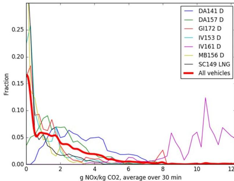
Figure 13: Frequency distribution of 30-min window average emissions of NO<sub>x</sub> for all test data combined. Vehicle IV161 is tested under worst case conditions which can't be regarded as representative, see paragraph 2.2.
