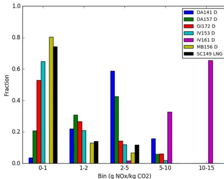
Figure 12: Frequency distribution of 30-min window average emissions of  $\text{NO}_x$  for all vehicles. 1 g  $\text{NO}_x/\text{kg CO}_2$  is comparable to 0.69 g  $\text{NO}_x/\text{kWh}$ . Vehicle IV161 is tested under worst case conditions which can't be regarded as fully representative, see paragraph 2.2.
