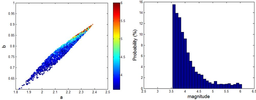
Figure 9: Scatterplot showing all  $a$ -,  $b$ - and  $M_{\max}$  values feasible for all induced earthquakes in the Netherlands between 1986 and 2010 (left) and the estimation of the maximum possible magnitude (right).
