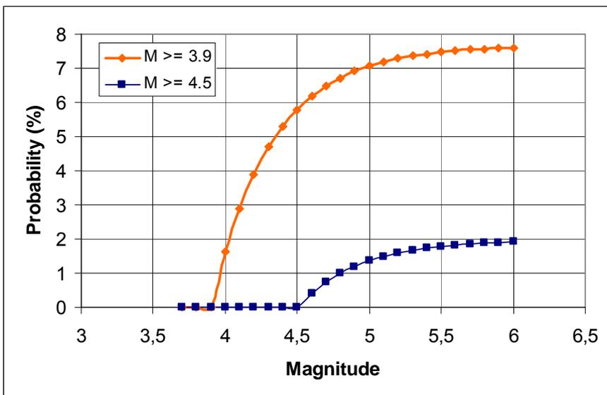
Figure 15: Expectation values for the probability of an earthquake of magnitude 3.9 or higher and 4.5 or higher, respectively, occurring in 2013 as a function of imposed maximum possible magnitude. The calculation is based on the expectation number of earthquakes predicted by equation (2) due to the already realised production rate between July 2011 and July 2012 and the cumulative production in July 2012, which results in an expectation value of 20 earthquakes of magnitude 1.5 or higher.
