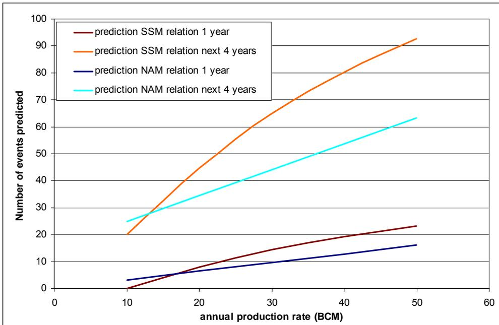
Figure 17: Comparison between the expectation number of earthquakes predicted by the NAM linear correlation and the SSM rate type compaction model based equation.
