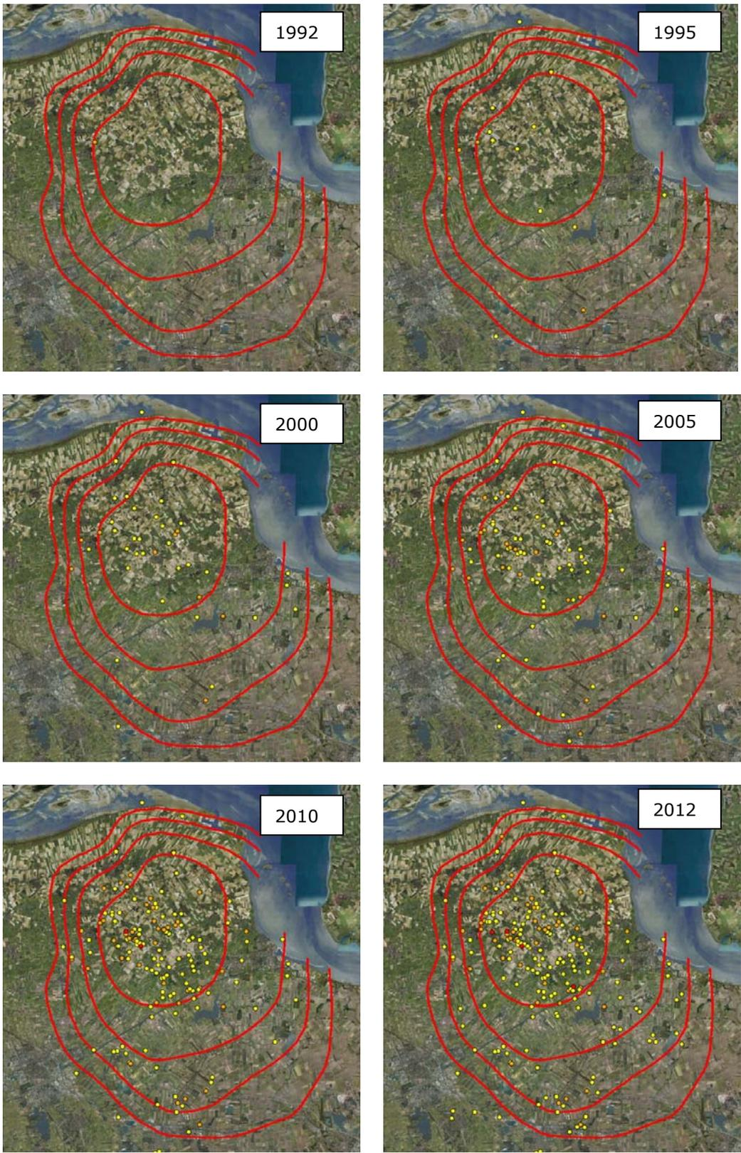
Figure 1: Spatial distribution of earthquakes over the Groningen gas field through time. The colour coding of the dots indicates the magnitude class: yellow  $1.5 \leq M \leq 2.0$ , orange  $2.0 < M \leq 3.0$ , red  $M > 3.0$ . The red lines indicate the contours of the subsidence bowl as observed in 2008.
