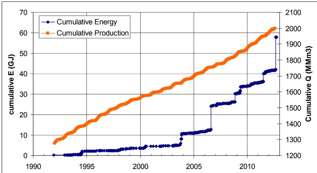
Figure 3: Cumulative seismic energy release and cumulative production through time. The higher magnitude earthquakes ( $M \geq 3.0$ ) release the most energy (10 times more than a magnitude 2.5 earthquake), which introduces the steps observed in the figure.
