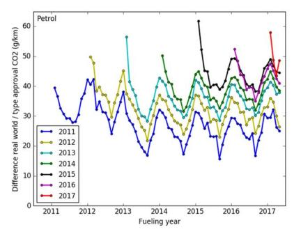
Figure 8: Evolution over time of the gap between real-world and type approval CO<sub>2</sub> emissions for petrol vehicles with different years of introduction in the Netherlands.
