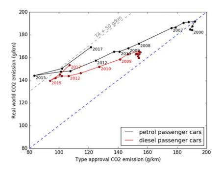
Figure SE1: Average real-world CO<sub>2</sub> emissions versus the average type approval value of new petrol and diesel cars, including plug-in hybrids, differentiated by the year of introduction / registration in the Netherlands (2017 value is preliminary)
