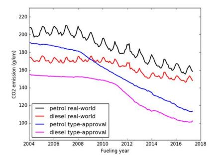
Figure 4: Average real-world and type approval tailpipe CO<sub>2</sub> emission of conventional and non-plug-in hybrid petrol and diesel vehicles in the database. Both the real-world and the type-approval CO<sub>2</sub> emissions have decreased since 2004. The different rates of reduction result in an increasing gap.
