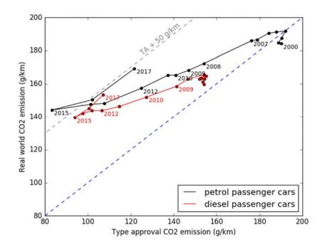
Figure 6: Average real-world CO<sub>2</sub> emissions versus the average type approval value of new petrol and diesel cars, **including plug-in hybrids**, differentiated by the year of introduction / registration in the Netherlands (data for 2017 are preliminary)
