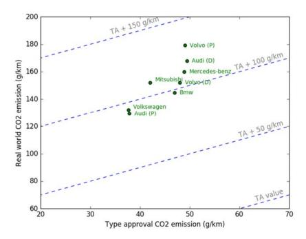
Figure 13: Average type approval and real-world CO<sub>2</sub> emission of **plug-in hybrid vehicles** sold in 2016 for the 10 top selling brands. P: petrol, D: diesel.
