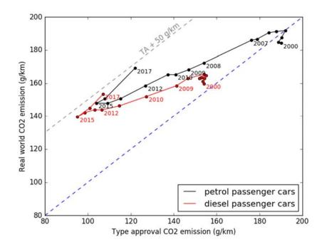
Figure 7: Average real-world CO<sub>2</sub> emissions versus the average type approval value of new petrol and diesel cars, **excluding plug-in hybrids**, differentiated by the year of introduction / registration in the Netherlands (data for 2017 are preliminary)
