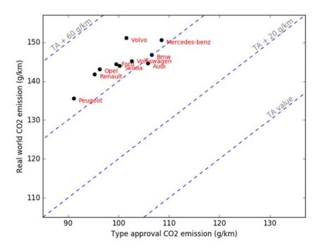
Figure 12: Average type approval and real-world CO<sub>2</sub> emission of **diesel vehicles** sold in 2016 for the 10 top selling brands. Plug-in hybrids are excluded.
