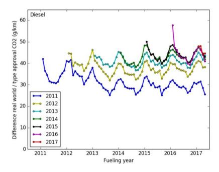
Figure 9: Evolution over time of the gap between real-world and type approval CO<sub>2</sub> emissions for diesel vehicles with different years of introduction in the Netherlands.
