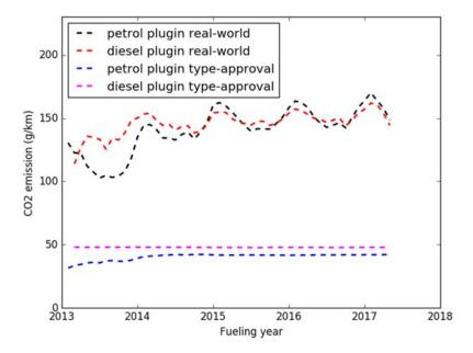
Figure 5: Average real-world and type approval tailpipe CO<sub>2</sub> emission of plug-in hybrid vehicles on petrol and diesel in the database. The real-world CO<sub>2</sub> emissions have increased since 2013, while the type-approval CO<sub>2</sub> emissions remained relatively constant. The increasing real-world emissions lead to an increasing gap.
