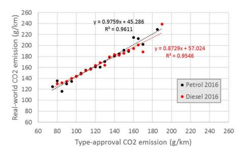
Figure 10: Correlation between absolute real-world CO<sub>2</sub> emissions and the average type approval value per segment, for new vehicles sold in 2016.
